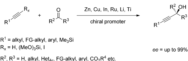
Scheme 124. Access to enantioenriched propargylic alcohols by catalytic enantioselective alkynylation of carbonyl compounds.
